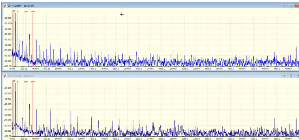
Figure 7: Gear Mesh Frequencies – December, 2016
