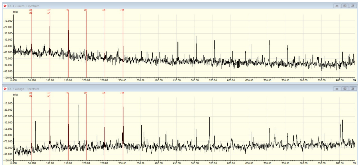
Figure 3: FFT of Voltage (bottom) and Current (top) with most of the expected peaks associated with inter-turn stress being low
