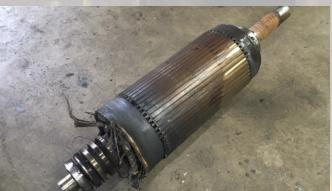
The motor failed within a few days of testing and it was found that one slip ring of the three had failed.
