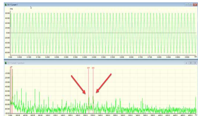
Fig. 4. Wedge signature in an 800 hp induction motor
