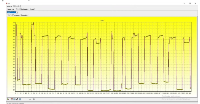
Figure 8: load profile in % of full load as set in the software header. Phase 3 issue shows during peak loads only.
