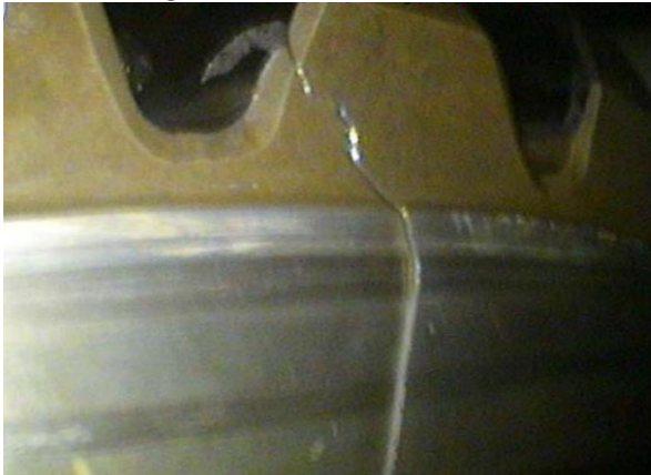
Figure 20: high speed wind turbine gear fracture.
