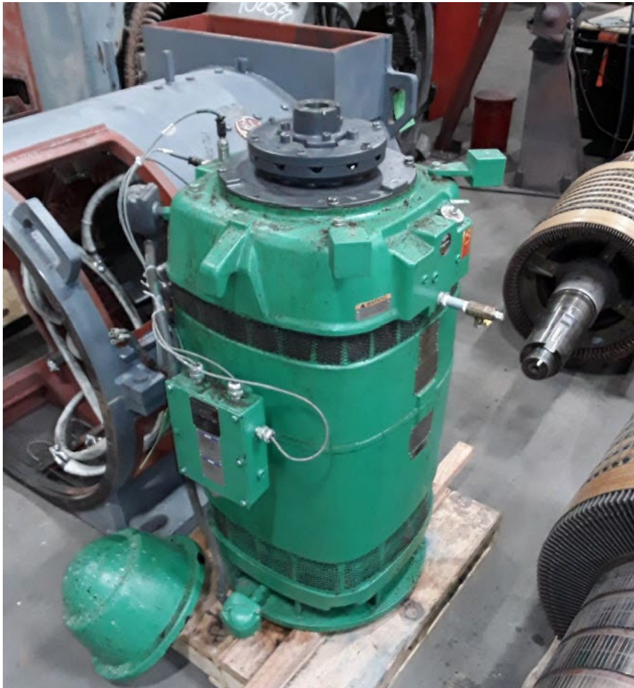
Figure 1: 350 horsepower electric motor prior to disassembly.
