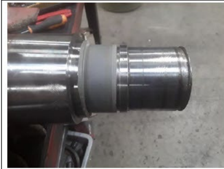
Figure 7: Removed bearing and bearing journal with ceramic.
