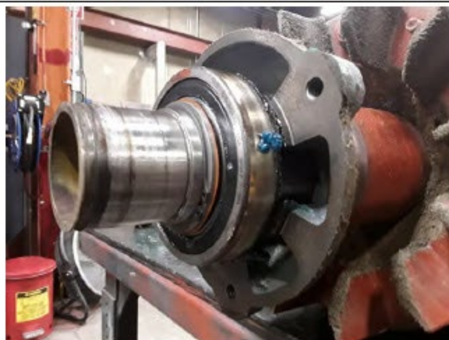
Figure 6: Drive end bearing - partial disassembly.
